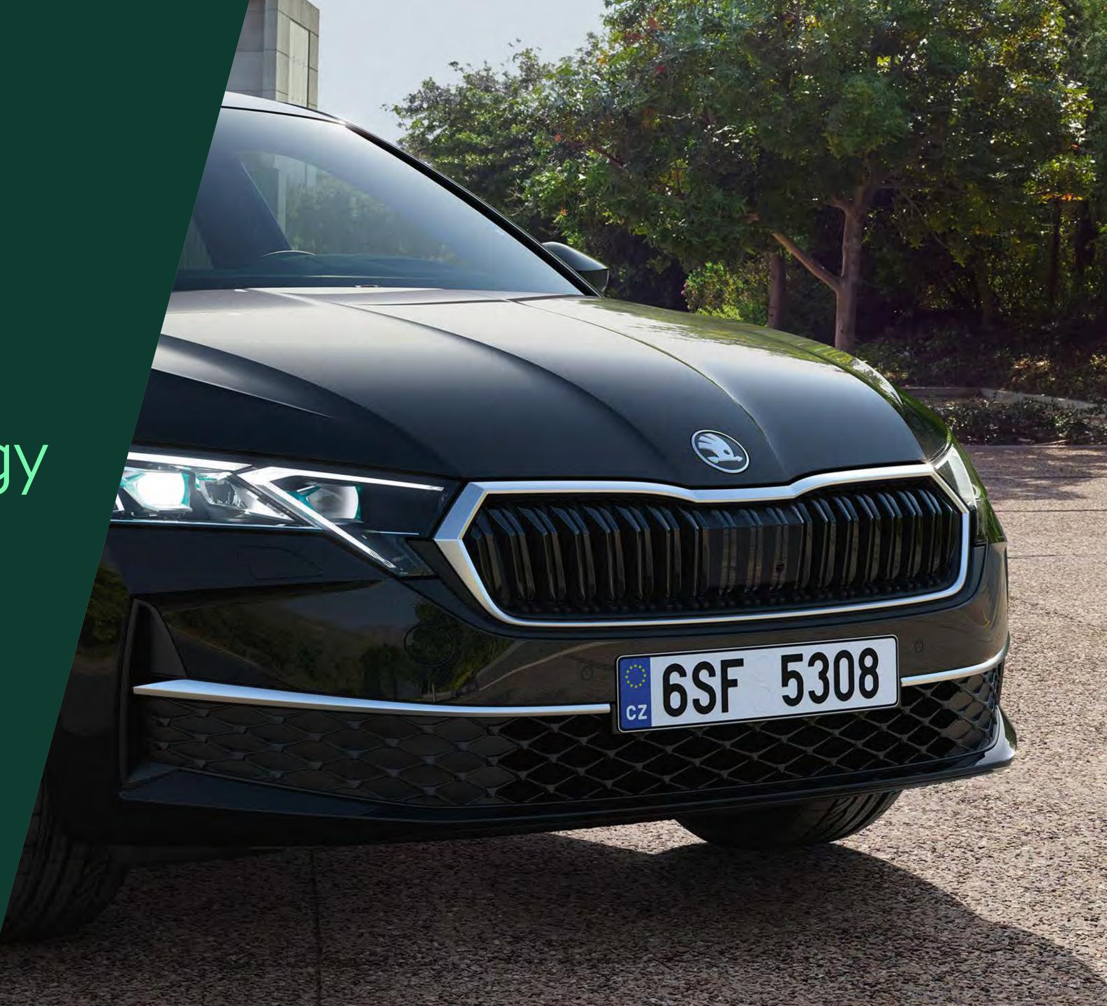
Middle East New aprons, front and rear, and a revised Škoda grille render a more modern styling for the Octavia. 36 individual matrix segments and new Crystallinium elements make up the advanced, second-generation LED Matrix beam headlights and deliver even better illumination of the road ahead while effectively shielding oncoming motorists from headlight glare.
