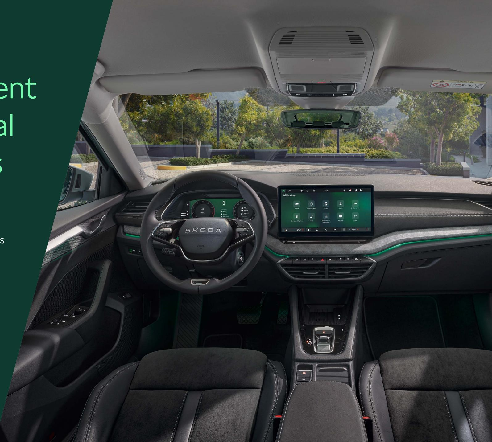
Middle East – For the first time ever, the Octavia is available with a 13-inch central infotainment display. USB-C ports, now rated at 45 Watts, offer more charging power. The Phone Box now also features more powerful wireless charging with a power output of up to 15 Watts and ventilation, while the 15-watt USB-C port on the back of the interior mirror remains for added functionality. All five interior Design Selections of the revamped Octavia benefit from increased use of sustainable materials.
