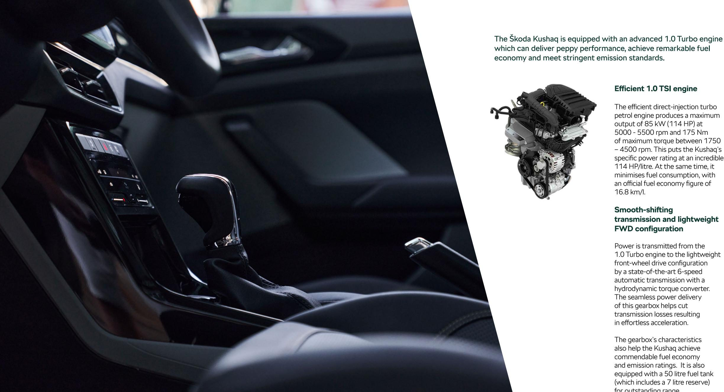
petrol engine produces a maximum output of 85 kW (114 HP) at 5000 - 5500 rpm and 175 Nm of maximum torque between 1750 – 4500 rpm. This puts the Kushaq's specific power rating at an incredible 114 HP/litre. At the same time, it minimises fuel consumption, with an official fuel economy figure of
