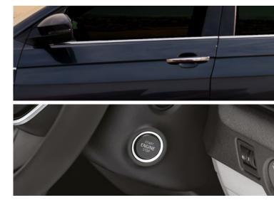
**Kessy** The Keyless Entry Start & Stop System enables convenient locking and unlocking of the car.
